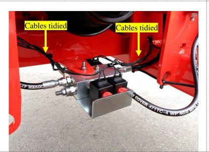
Tidy away the Hydraulic Valve Bank cables as shown.
