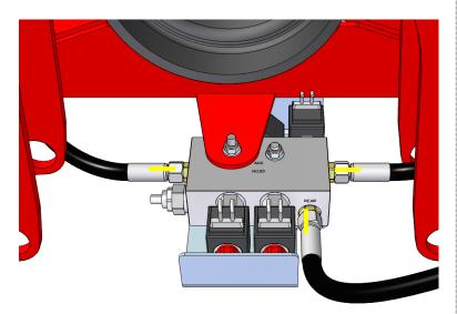
Reconnect the four Hydraulic Hoses to their relevant ports on the Valve Bank Assembly.
