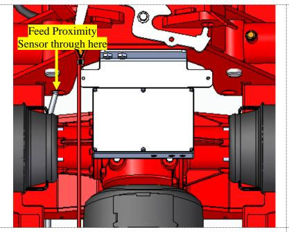
Remove the Nuts from the **REAR** Proximity Sensor.
