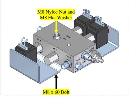
Offer up the Mounting Bracket (418-000-398) to the BOTTOM of the Valve Bank.
