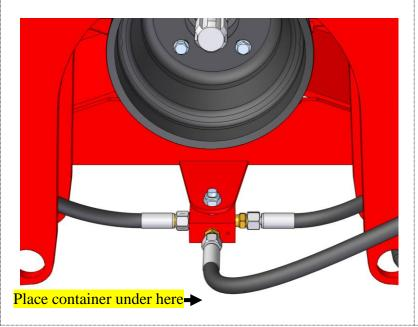
Place a suitable Container underneath the 4-Way Hydraulic Block (408-448-500)
