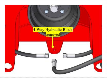
Disconnect the Hydraulic Hoses completely from the 4-Way Hydraulic Block.
