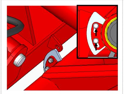
Right-hand QuikLIFT Cam Using 2x M6x16, 2x M6 Spring Washer and 2x M6 Flat Washers, position prox cam as shown in the insert.
