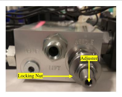
Once adjusted, use a 4mm Allen Key to hold the Adjuster stationary.
