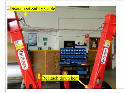
Disconnect the Safety Cable from Right-Hand Outrigger Arm.
