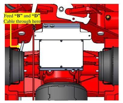
Identify the two Cables labelled "B" and "D" attached to the Command Module.
