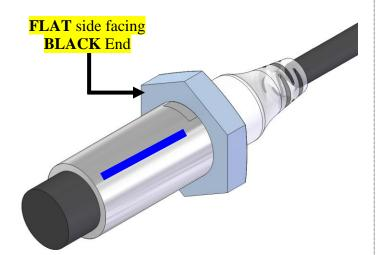
Apply Loctite 243 to the thread on the Proximity Sensor.
