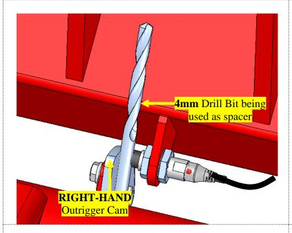
Set the **BLACK** end of the Proximity Sensor **4mm** away from the Cam on the Outrigger Arm.
