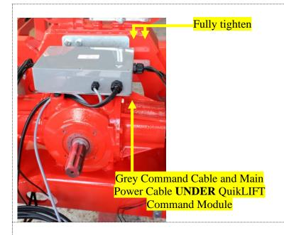
Pass the Grey Command Cable and the Main Power Cable **UNDER** the Right-Hand Side of the QuikLIFT Command Module as shown.
