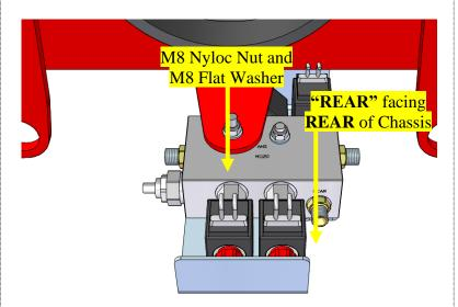
Offer up the Valve Bank Assembly to the Hydraulic Block Mounting Tag on the Pegasus Chassis.
