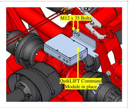
Offer up the QuikLIFT Command Module (505-000-008) to the TOP of the 4-Way Gearbox.
