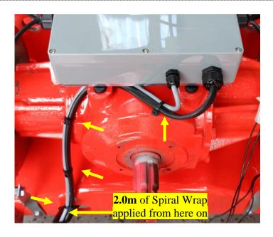
Secure the Command Cable and the Main Power Cable together using four Cable Ties in the locations shown.
