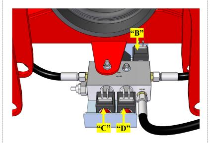
Plug the four Cables (**B, C** and **D**) into their respective Plugs present on the Hydraulic Valve Bank.
