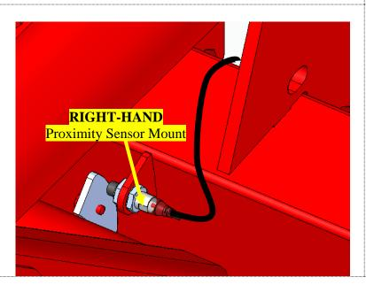
Pass the **BLACK** end of the Sensor through the **RIGHT-HAND** Proximity Sensor Mount as shown.
